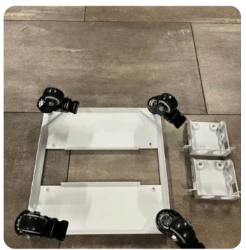
**Step 3:** Flip the stand onto its casters and install the 2 side braces and tighten using the provided screws with a Philips head screwdriver. (Ensure the holes line up as shown in the picture)
